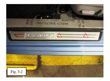
3. Install front left (driver side) and front right (passenger side) door sill enhancements.
