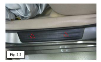
(b) Remove the rear left and rear right door scuff plates using a nylon panel removal tool to disengage the 2 clips. (Fig 2-2)
