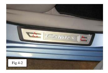
4. Install rear left (driver side) and rear right (passenger side) door sill enhancements.
